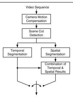
**Figure 1** Video segmentation framework in Annex-F of MPEG-4 standard.
