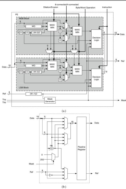
switches (multiplexers) for a 9-bit MSB channel (MSB 9-bit of *Data*), a 9-bit LSB channel (LSB 9-bit of *Data*), and an 8-bit reference channel. Referring to the instructions described in Fig. 9b, for the MSB channel, the output of the routing switch could be the original MSB data (*ORI*), the LSB data (swapped data, *SWP*), the
