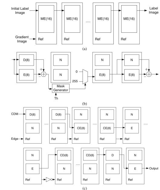
Figure 13 Example of different configuration for different operations: a watershed; b edge detection; c edge fitting.
