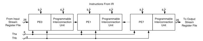
Figure 11 Architecture of programmable PE array.
