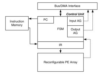
Figure 10 Detailed signals to be controlled by Control Unit.
