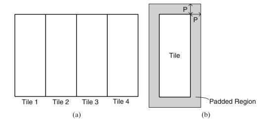
of morphological operations can be handled well without complicated control circuits. After all the tiles are processed, the result is the same as when the whole frame is processed at the same time; however, the length of the delay line becomes about a quarter of the original one, and three-fourths of the hardware cost can be saved. The overhead of the tiling technique is the increasing complexity of addressing and the longer latency because of the padded regions.
