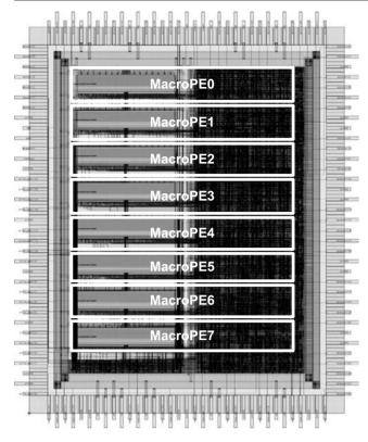
Figure 20 Layout of the prototyping chip.
